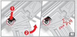
Let a magazine be attached with the magazine release lever (step 2) until set firmly.
