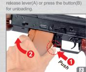
Hold the magazine, push the magazine release lever(step 1) for unloading.
