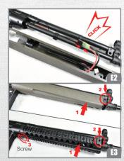
Connect the battery. Attach the handguard by steps.
