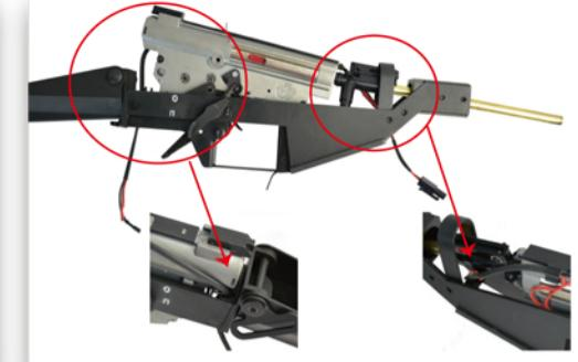
1. Install Hop-Up chamber and gear box.
