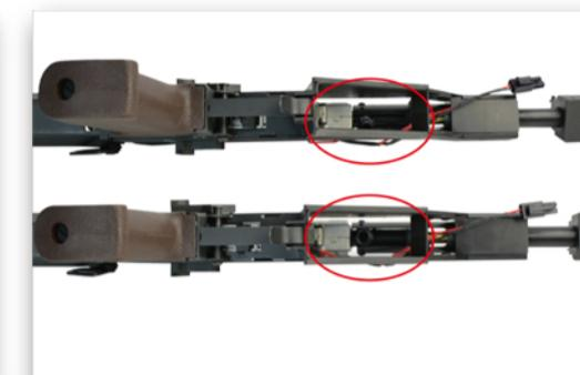
2. First, secure the gearbox screws, then install the gearbox wires onto the motor. The red wire should attach to the red connector and black wire to the silver connector, then tighten the motor screws.
